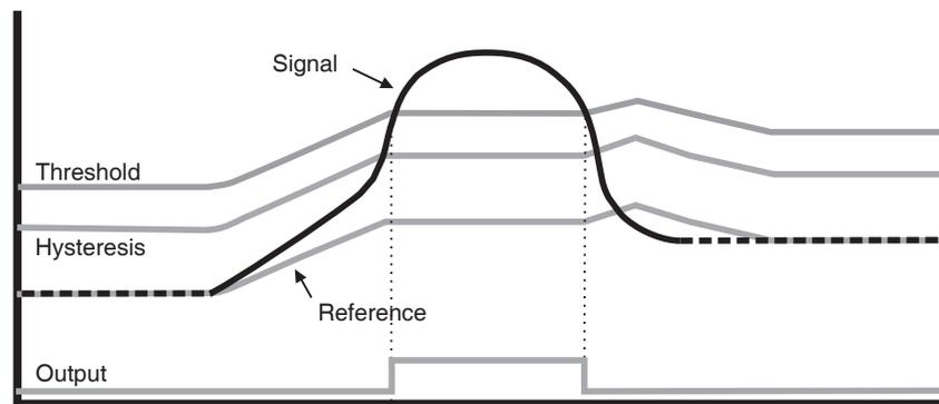
The device drift compensates using a slew-rate limited change to the reference level; the threshold and hysteresis values are slaved to this reference.
