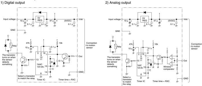
Note: This is the reference circuit which drives the PIR motion sensor. Install a noise filter for applications requiring enhanced detection reliability and noise withstanding capability.
