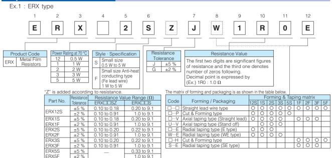
The above example 1 shows a small metal film resistor, 2 W power rating, resistance value of 1.0  $\Omega$ , tolerance ±5 %, and package of radial taping
