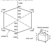
**Test Conditions:** Shock is applied in  $\pm X$ ,  $\pm Y$ ,  $\pm Z$  directions three times each with and without energizing the relays to check the number of malfunctions.
