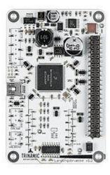
The "Landungsbrücke" is the connection between your desktop computer and Trinamic's Chip solutions. Just connect the desired board combination and start to discover Trinamic's unique features.
