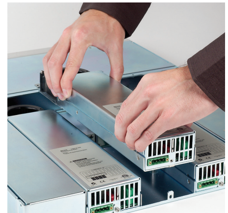
Figure 6c. User re-configurable modular system
